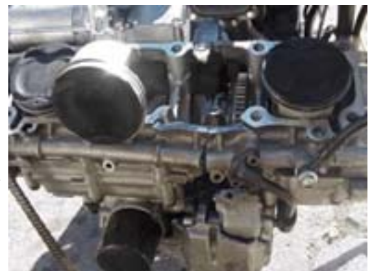
A wrist pin/rod failure can destroy the whole motor.
